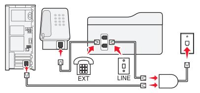
A Digital Subscriber Line splits your regular telephone line into two channels: voice and Internet. Telephone and fax signals travel through the voice channel, and Internet signals pass through the other channel. This way, you can use the same line for analog voice calls (including faxes) and digital Internet access.
